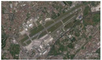
The airport has a single runway (orientation: 06/24) 2,628 m × 45 m in bituminous conglomerate and concrete, with one taxiway. There is one apron with 29 stands, 9 of which self-maneuvering and the remaining Push Back. The airport is class 4D ICAO and has the classification of military airport opened to commercial air traffic 24 hours/day.
